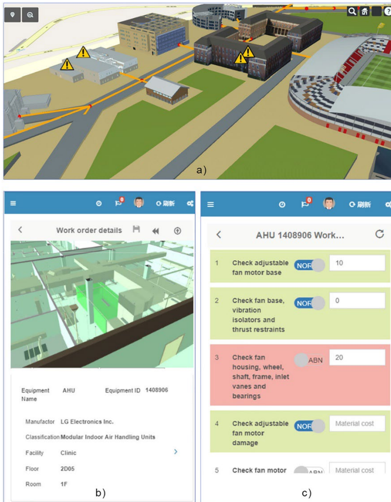
Figure 5 BIM-based system for managing maintenance work orders
